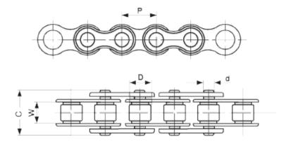
$\begin{array}{lll} \text{Breaking power} = 31800 \\ \text{C} & = 25,90 \\ \text{Chain size} & = 3/4" \\ \text{d} & = 5,94 \\ \text{D} & = 11,91 \\ \text{Description} & = 60 \\ \text{P} & = 19,050 \\ \text{W} & = 12,57 \\ \end{array}$
